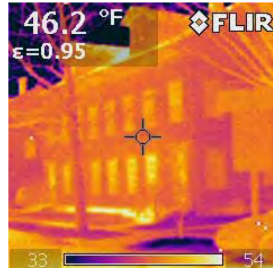
An infra-red image of one of the buildings showing greater heat loss at the windows.
